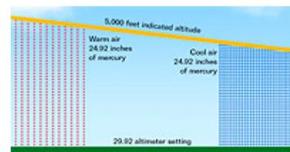
Figure 3: How differences in temperature affect indicated altitude.
